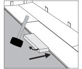
Step 5: IMPORTANT! Use hammer and tapping block to tap long edge of plank to ensure a tight fit. ANY GAPPING CAN COMPROMISE THE LOCKING SYSTEM!
