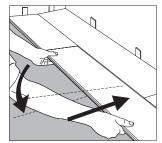
Step 4: Lock long edge of plank by inserting tongue into groove and drop in place.
