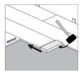
Step 7: Tap end of plank with hammer and tapping block to lock ends of planks together. Remove bridge and continue towards wall until installing the final plank in the row. BE SURE TO TAP ON EDGE OF VINYL SO AS NOT TO DAMAGE LOCKING PROFILE.
