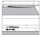
**Step 3:** Use leftover plank from first row as starter for second row. There must be at least 300mm between plank end joints on adjacent rows.
