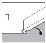
Step 2: Lock short end of plank by tapping down the ends until they lock into place. Continue to end of first row.
